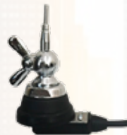
MA-1301 VHF, 140÷ 174 MHz, 1/4 λ, 2.14dBi, 5 m cable
